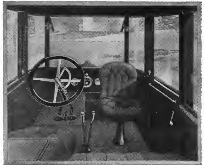
Interior view of Overland coupé. The entire interior is finished in Bedford cloth. Levers operate the windows, foot pedals are adjustable and all passengers face forward. This car sells for $1,600
